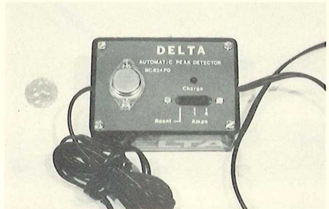
The Delta Charger automatically cuts off charge at peak battery capacity.
